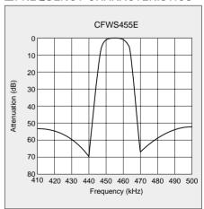
Note: To take best advantage of safety feature of ceramic filters, connect the output to an IF amplifier through a DC cut capacitor. Avoid directly applying a direct current to output of ceramic filters (between ⑤ and ②,③,④).
